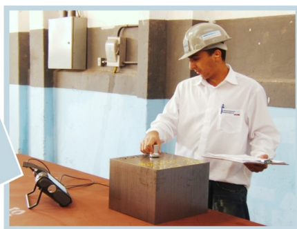
Ultrassom Mentor UT Waygate (GE), Software: Mentor Create, Sistema: Linux 4.7.2
