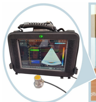
Ultrassom Mentor UT Waygate (GE), Software: Mentor Create, Sistema: Linux 4.7.2
